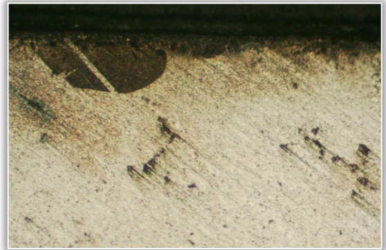
Plate 5. Optical micrographs of samples oxidized at 1050°C for 10 hours (a) Haynes 282 Sample 4 (100x), (b) Inconel 718 Sample D (100x)
