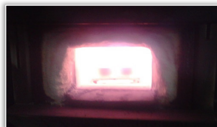
Figure 1. Experimental Setup: (a) sample arrangement inside the crucible; (b) crucible arrangement in the furnace; (c) furnace stability at first test temperature; (d) furnace environment before samples were retrieved
