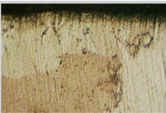
Plate 8. Optical micrographs of samples oxidized at 1100°C for 8 hours (a) Haynes 282 Sample 7 (100x), (b) Inconel 718 Sample G (100x)
