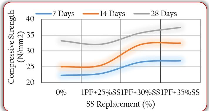
Figure 2: Compressive Strength of Concrete Grade 30 (Kumar and Kumar, 2016)
