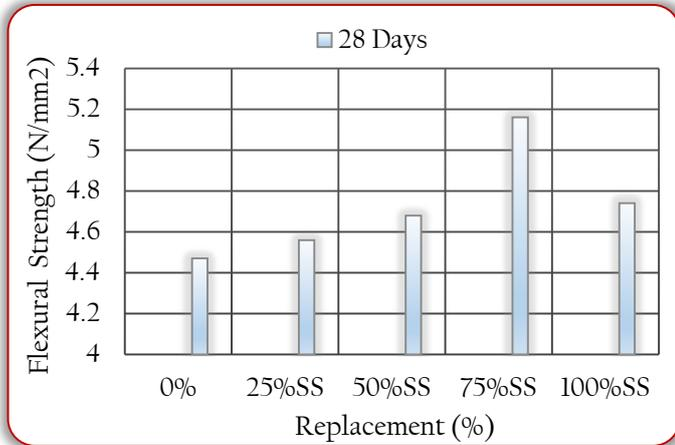
Figure 16: Flexural Strength of Concrete Using Steel Slag (Warudkar and Nigade, 2015)
