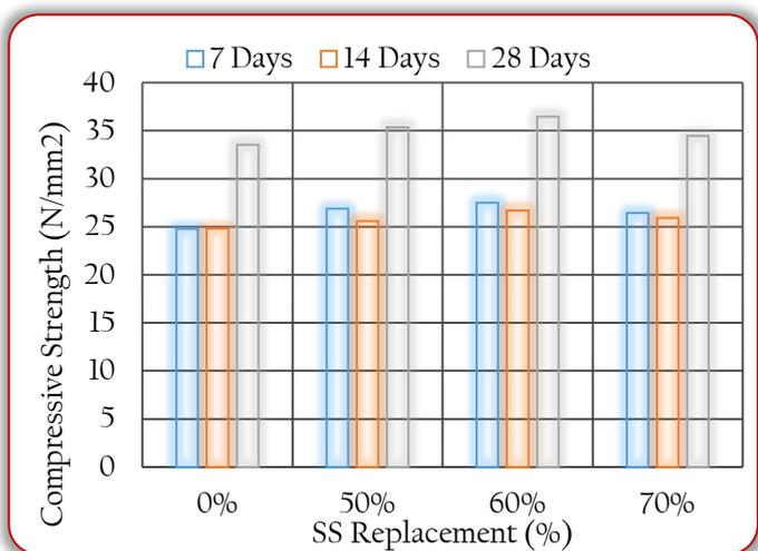
Figure 5: Compressive Strength Vs Steel Slag Concrete (Subramani and Ravi, 2015)
