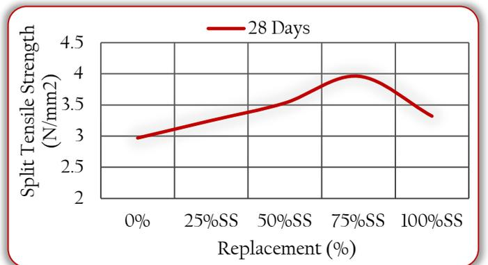
Figure 11: Split Tensile Strength of Concrete at 28 Days Curing (Warudkar and Nigade, 2015)
