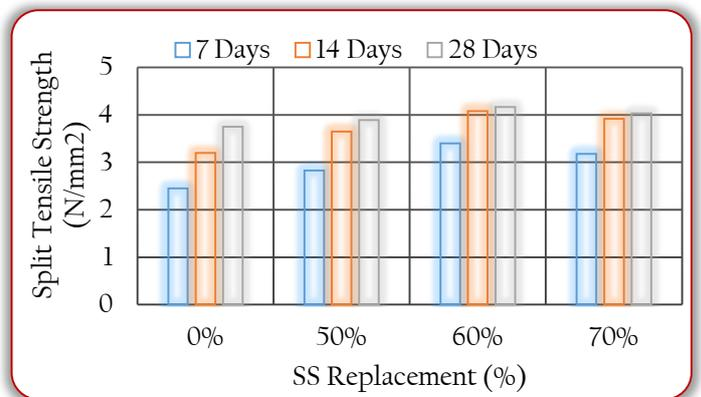
Figure 10: Split Tensile Strength against Steel Slag Concrete (Subramani and Ravi 2015)
