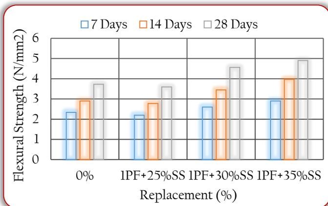
Figure 12: Flexural Strength of Concrete (Kumar and Kumar, 2016)
