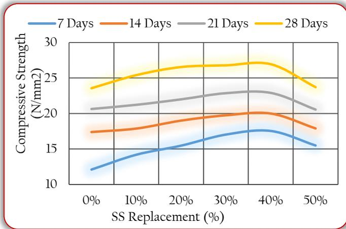
Figure 7: Graphical representation of Compressive Strength against SS Replacement (Anifowose *et al.*, 2017)
