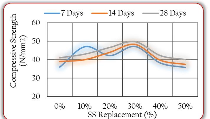
Figure 3: Steel Slag Compressive Strength (Raza *et al.*, 2014)
