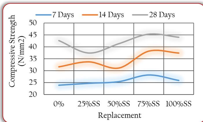
Figure 6: Compressive Strength of Concrete (Warudkar and Nigade, 2015)
