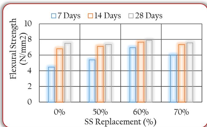
Figure 15: Flexural Strength Vs Steel Slag Concrete (Subramani and Ravi 2015)
