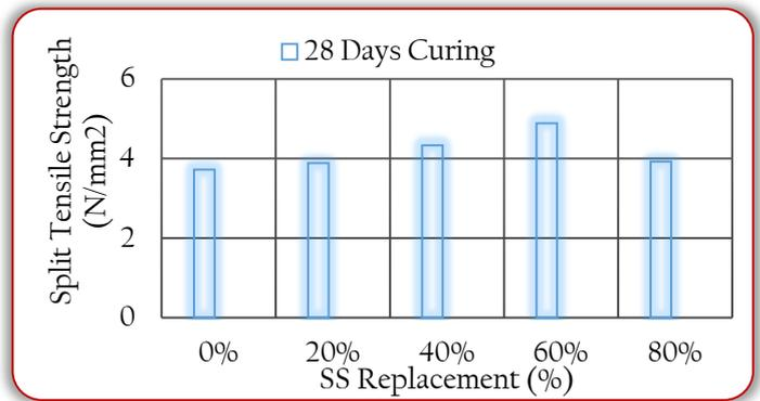
Figure 9: Split Tensile Strength of Steel Slag Concrete (Thangaselvi, 2015)
