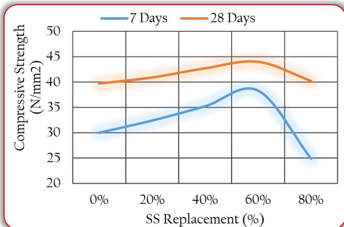
Figure 4: Compressive Strength of Steel Slag Concrete (Thangaselvi, 2015)
