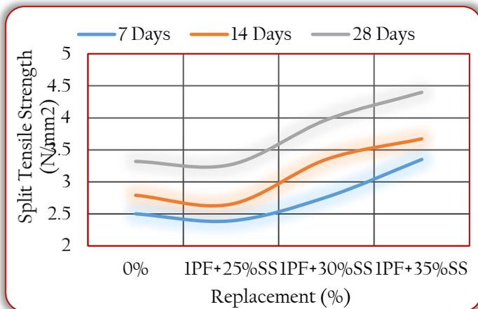
Figure 8: Split Tensile Strength for Concrete Grade 30 (Kumar and Kumar 2016)
