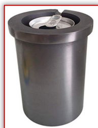
Figure 9. Micro station for melting of aluminium wastes from the beverage cans: (a) the melting aggregate; (b) the crucible
