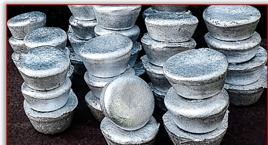
Figure 11. Casting of recovered aluminium wastes from the beverage cans: (a) ingots casting; (b) aluminium ingots
