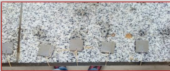
Plate 4: Cleaned specimen after corrosion test
