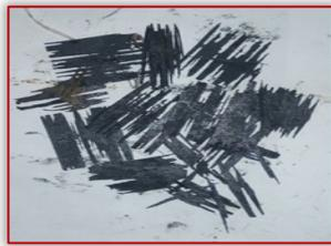
Plate 7: AISI 1007 steel that could not withstand beyond 336 hours
