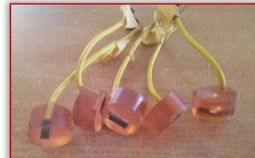
Plate 6: Coupons after TAFEL Polarization test
