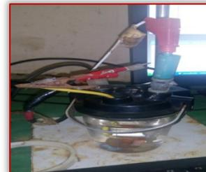
Plate 5: Electrochemical Measurement (TAFEL Polarization set-up)
