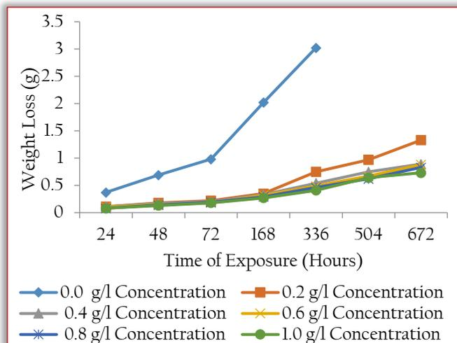
Figure 1: Variation of weight loss with time for the corrosion of AISI 1007 Steel in 2M HCl with and without inhibitor (peel extract)
