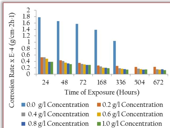
Figure 2: The variation of Corrosion rate in cucumber peel extracts
