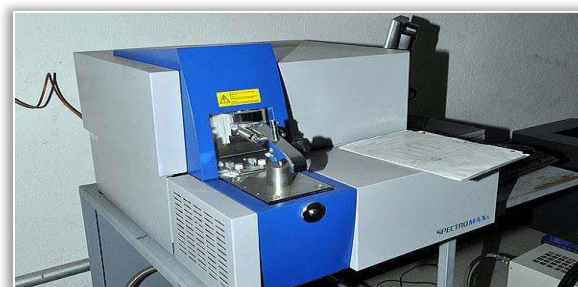
Figure 3: Determining the chemical composition of analysed samples [4]
