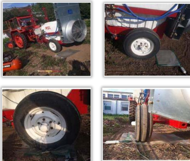
Figure 1 – Field testing of the MSL spraying machine
