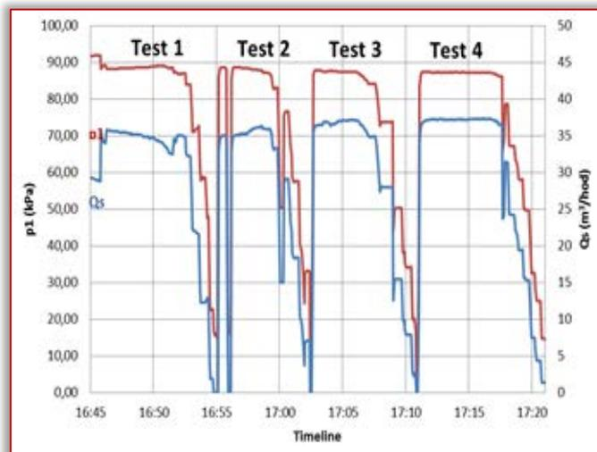
Figure 3: Measured values of absolute pressure and sucked air in vacuum pump suction
