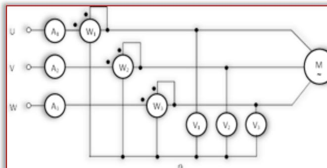
Figure 4: Scheme of measuring the electric input.
