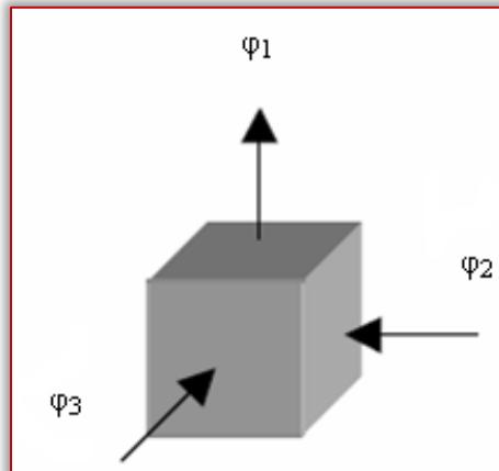
Figure 3: Principal schemes of elementary bulk deformation
