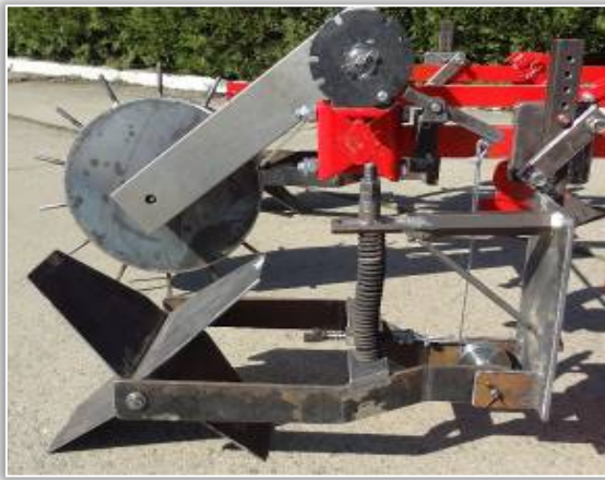
Figure 4 – Device of forming compartmented furrows Mechanism of command (Figure 5) comprises: spur wheel, a transmission system and a driving mechanism.
