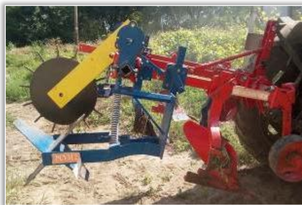
Figure 3 – Equipment for soil modelling in compartmented furrows in vine and tree plantations, simultaneously in two furrows in the same space, PCVM2,2+EMBC2-0
