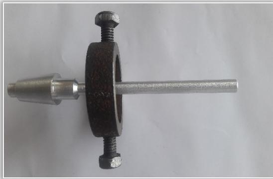
Figure 3: Fretting arrangement
