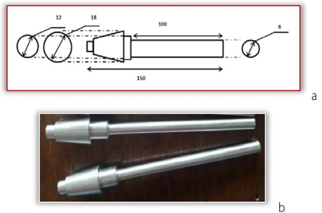
Figure 1: Designed specimen (dimensions are in mm) (a), prepared Specimens (b)
