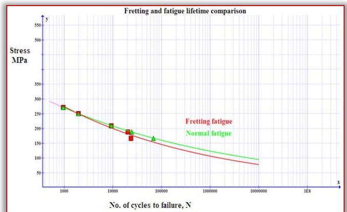
Figure 7: Comparison of fretting fatigue lifetime with normal fatigue
