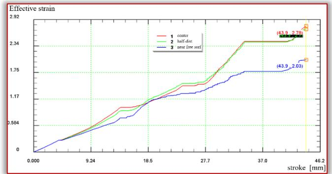
Figure 5. Effective strain distribution at sample cross-section in three different locations
