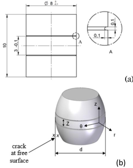
Figure 4. Cylinder dimensions (a) and crack at free surface (b)
