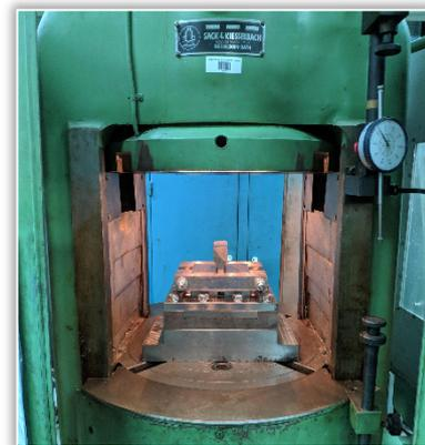
Figure 2. Plane strain compression die mounted on hydraulic press
