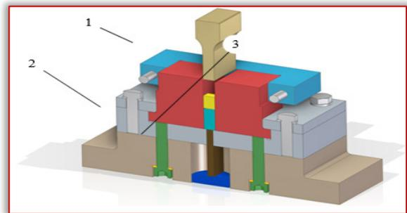
Figure 1. Section of the die CAD model; 1 - punch, 2 - mould, 3 - sample
