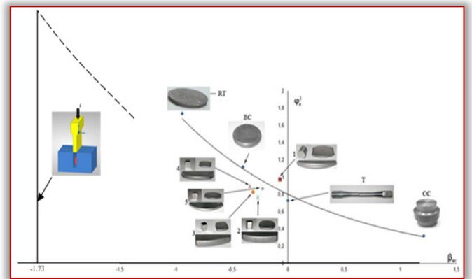
Figure 6. The position of Plane strain compression process in workability diagram [20]
