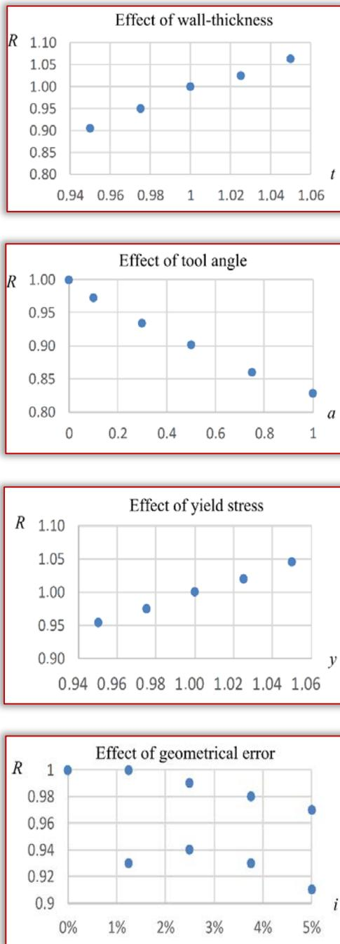
Figure 4. The effect of some properties on the buckling load
