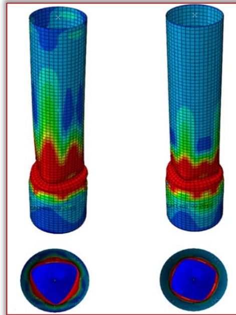
Figure 5. Possible buckled shapes with some imperfections introduced (magnified deformations)
