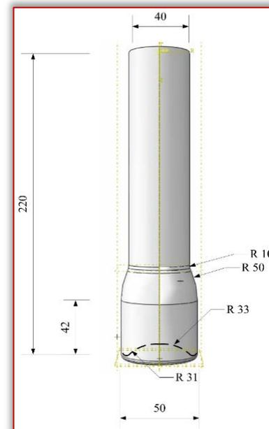
Figure 1. The initial geometry of the can
