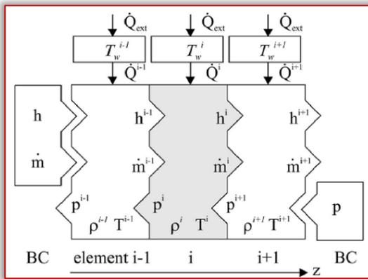
Figure 4. Axial discretization of fluid and pipe sections [20]
