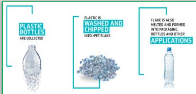
Figure 14. Recycling PET waste into new bottles
