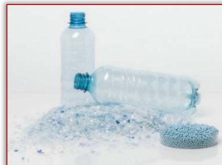
Figure 12. PET waste and crushed PET flakes
