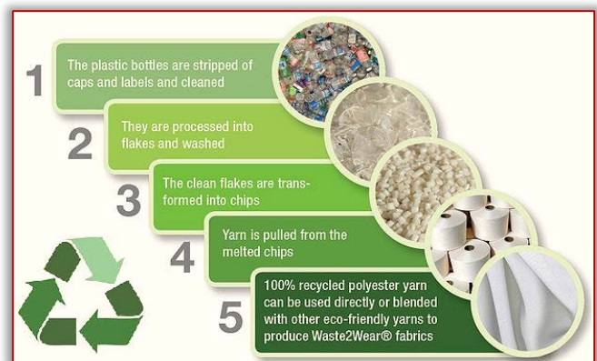
Figure 13. Recycling PET waste into polyester fibres
