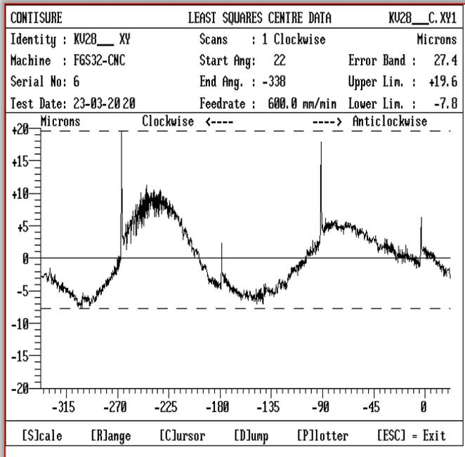
Figure 4. Linear diagram of the results of a measured circular test (feedrate  $v=600$  mm/min, radius of the circle  $R=150$  mm, position loop gain  $Kv=28.3$  s<sup>-1</sup>,  $a=0$ , clockwise direction)
