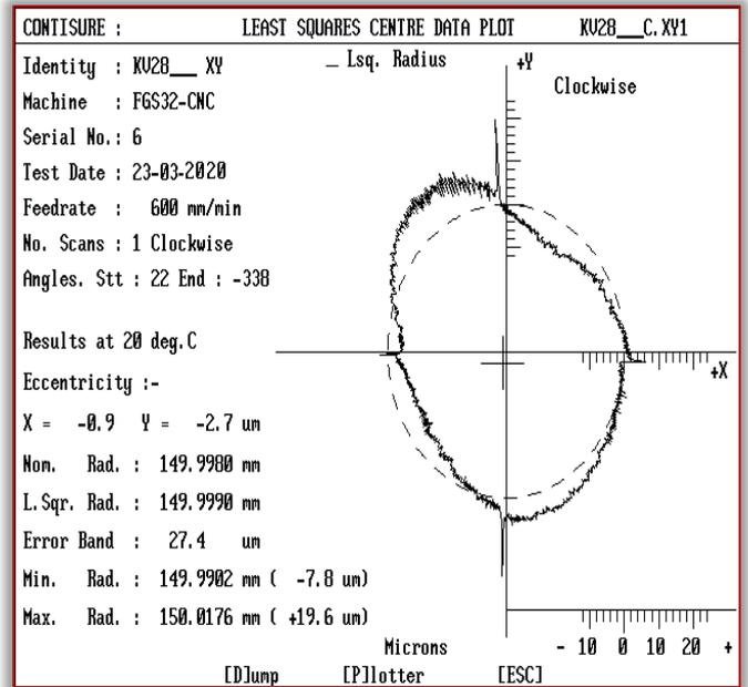
Figure 2. Polar diagram of the results of a measured circular test (feedrate  $v=600\text{ mm/min}$ , radius of the circle  $R=150\text{ mm}$ , position loop gain  $Kv=28.3\text{ s}^{-1}$ ,  $a=0$ , clockwise direction).
