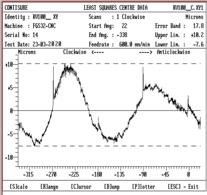
Figure 5. Linear diagram of the results of a measured circular test (feedrate  $v=600$  mm/min, radius of the circle  $R=150$  mm, position loop gain  $Kv=100$  s<sup>-1</sup>,  $a=0$ , clockwise direction)
