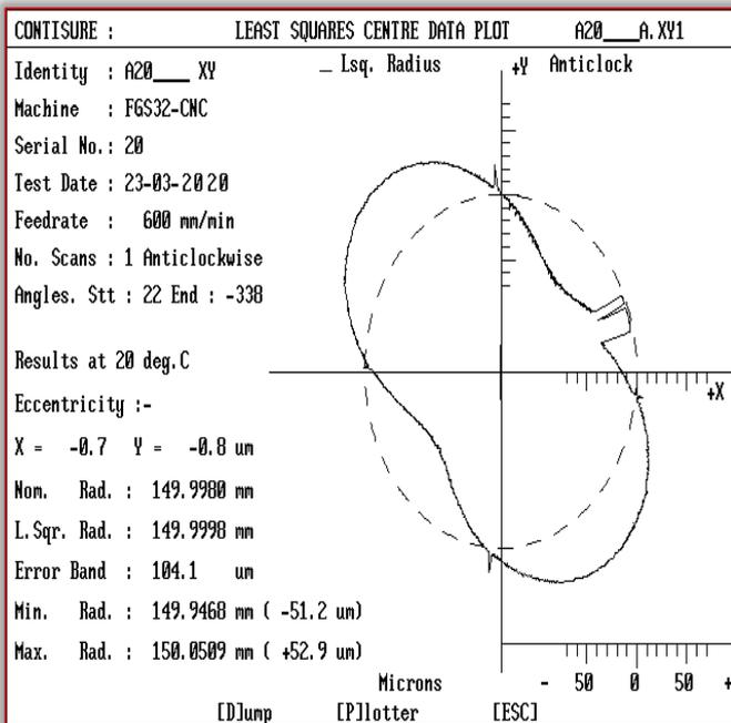
Figure 7. Polar diagram of the results of the measured circular tests with gains mismatched  $a=20\%$  (anticlockwise direction, feedrate  $v=600$  mm/min, radius of the circle  $R=150$  mm, position loop gains  $K_{vx}=30$  s<sup>-1</sup> and  $K_{vy}=24$  s<sup>-1</sup>)
