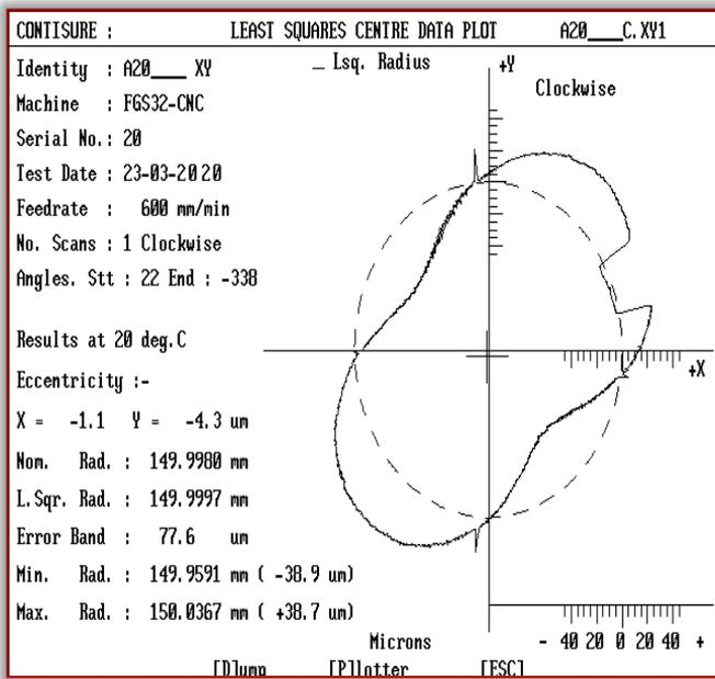
Figure 6. Polar diagram of the results of the measured circular tests with gains mismatched  $a=20\%$  (clockwise direction, feedrate  $v=600$  mm/min, radius of the circle  $R=150$  mm, position loop gains  $K_{vx}=30$  s<sup>-1</sup> and  $K_{vy}=24$  s<sup>-1</sup>)
