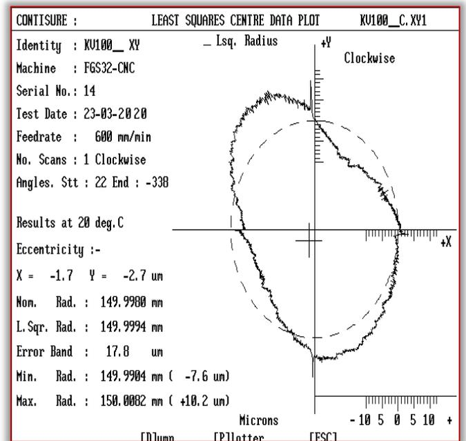
Figure 3. Polar diagram of the results of a measured circular test (feedrate  $v=600\text{ mm/min}$ , radius of the circle  $R=150\text{ mm}$ , position loop gain  $Kv=100\text{ s}^{-1}$ ,  $a=0$ , clockwise direction)
