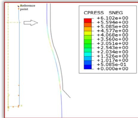
Figure 4. The assembly of the second method and the contact pressure during the forming process
