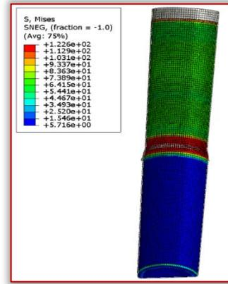
Figure 3. The deformed finite element mesh of the first example (with the von Mises stress distribution)
