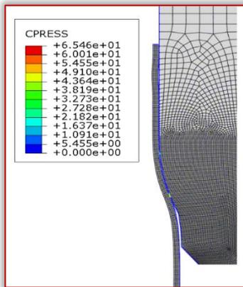
Figure 7. The contact pressure with deformable tool
