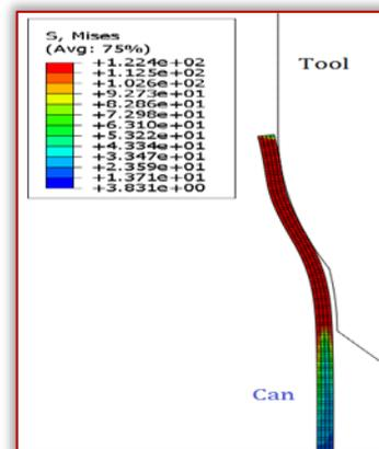
Figure 5. The deformed mesh of the first example using rigid tool and deformable can
