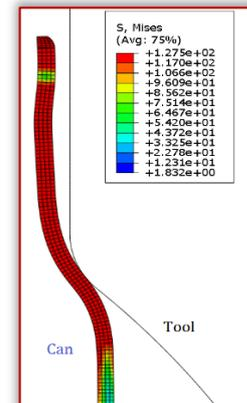
Figure 10. The deformed mesh of the second problem modelled with axisymmetric solid element and rigid tool
