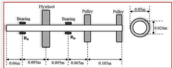
Figure 2: Schematic diagram of loads on the shaft
