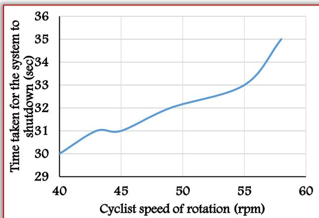
Figure 3: Graph showing relationship between the cyclist speed and time taken before the system shutdown
