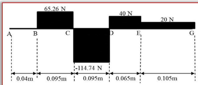
Figure 4: Shear force diagram for the shaft
