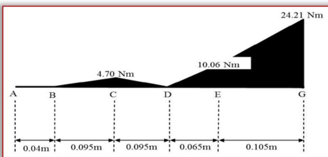
Figure 5: Bending Moment diagram for the shaft
