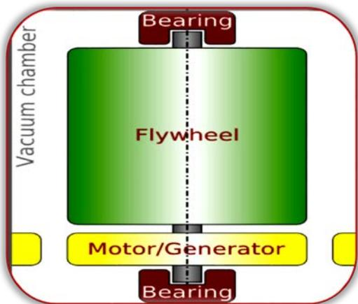
Figure 1: Schematic diagram for a flywheel’s storage system [8]
