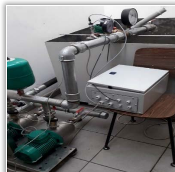
Figure 4. Testing the injection device with differential piston under laboratory conditions
