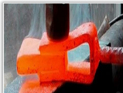
Figure 4. Critical moments in hand forge welding: a) beginning (bright color) and b) at the end (pieces were cooled to orange color)
