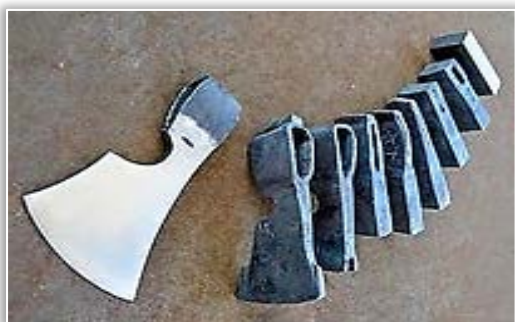
Figure 6. Some steps in hand forging/forge welding of an axe with insert of high carbon steel
