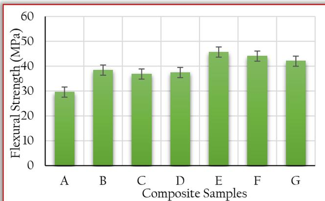
Figure 2: Flexural strength of the composites
