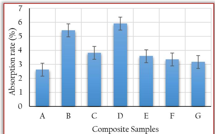
Figure 4: Water absorption rate of the composites
