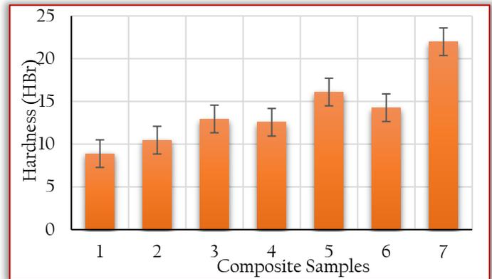
Figure 3: Hardness of the composites
