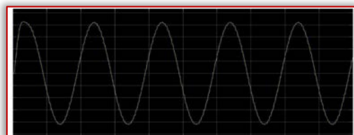
Figure 20. Inverter output after passing through Filter
