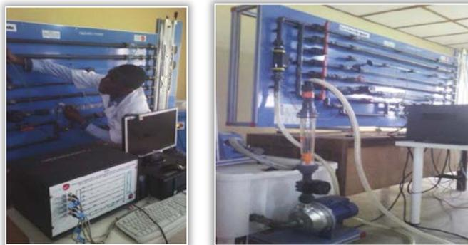
Figure 2: Fluid Friction Factor Board Set Up for Venturi Tube Meter
