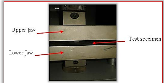
Figure 4: Compression test of test specimen
