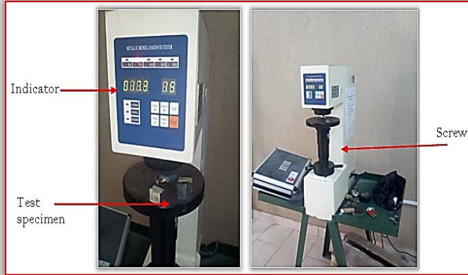
Figure 1: Brinell hardness test of test material
