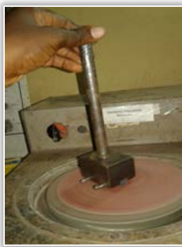
Figure 6: Test specimen under wear test
