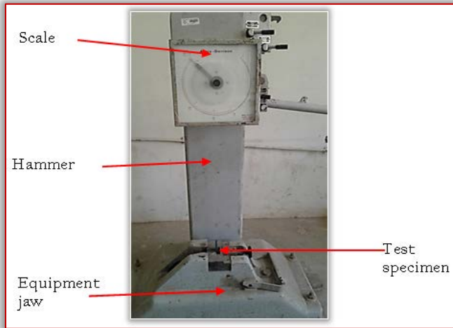
Figure 2: Izod impact test on test specimen
