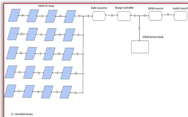
Figure 1. PV Model Under Case Study Showing Identified Nodes
