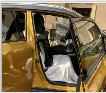
Figure 3. Placement of the psychoacoustic head in the vehicle
