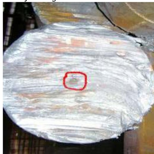
Fig. 12. Shrinkage cavity
