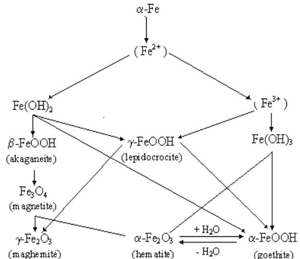
Figure 2 - Hiller scheme for the iron rust compounds [12] In the first phase of the steel rusting forms  $Fe(OH)_2$ , which it oxidizes suddenly forming lepidocrocite ( $\gamma$ - $FeOOH$ ), a crystalline phase with rhombic structure. In function of water presence or absence, this isomerises in goethite ( $\alpha$ - $FeOOH$ ), with rhombic structure also. If the corrosion rate is low, a part of lepidocrocite it transforms in maghemite ( $\gamma$ - $Fe_2O_3$ ), having a cubic structure.
