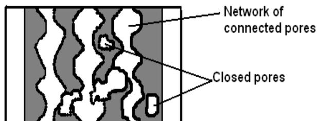
Figure 1. Schematic representation of an acoustical porous medium [9]
