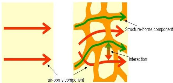
Figure 5. The sound propagation in the air (left) and in a porous material (right)[10]
