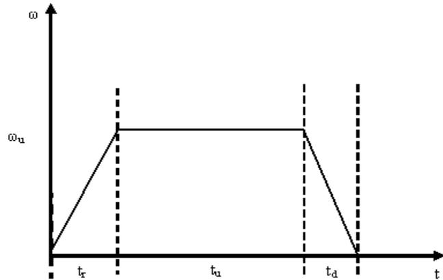
Figure 4. Trapezoidal velocity profile, length start  $\varphi_r = k_1 \cdot \varphi$ ; length end  $\varphi_h = k_1 \cdot \varphi$
