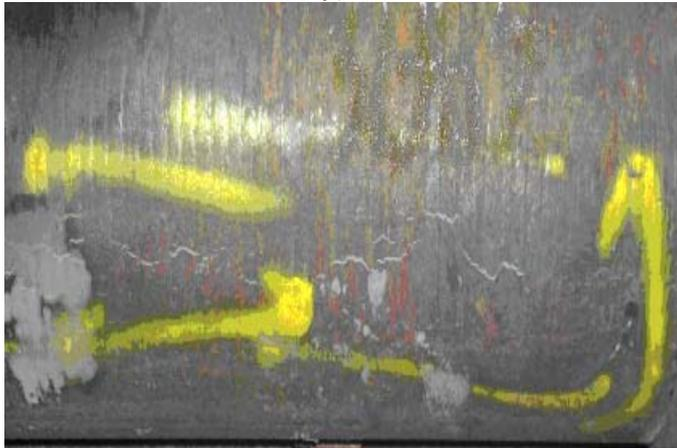
Fig. 7. Star cracks
