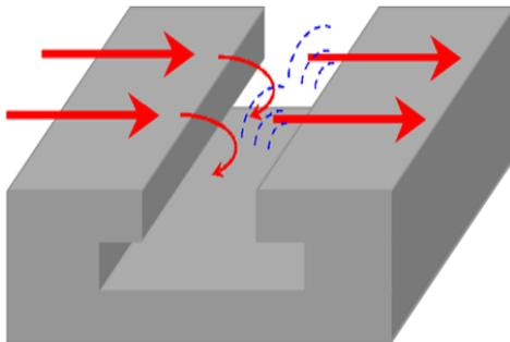
Figure 6. Flowinf of sound in hollow spaces [3]
