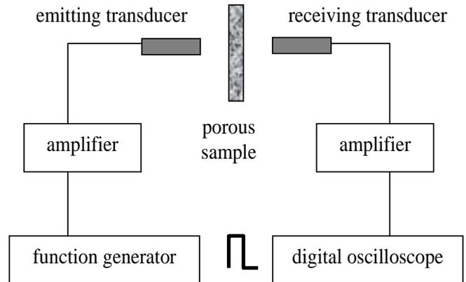
Figure 6. Schematic representation of the tortuosity measurement apparatus [11]
