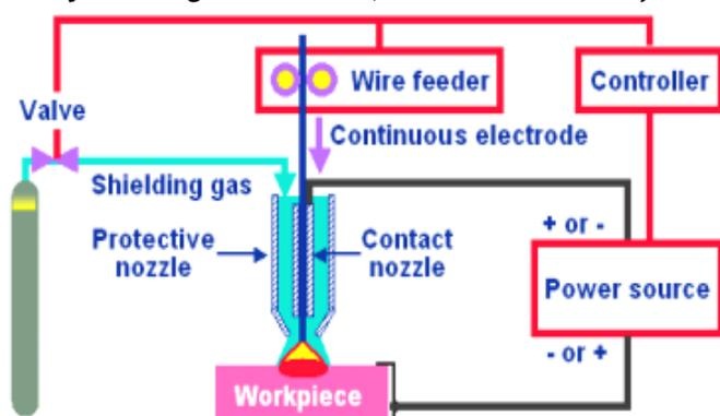
Fig. 2. MIG / MAG welding process
