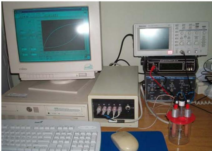
Figure 1. Photograph of the electrochemical measurement system
