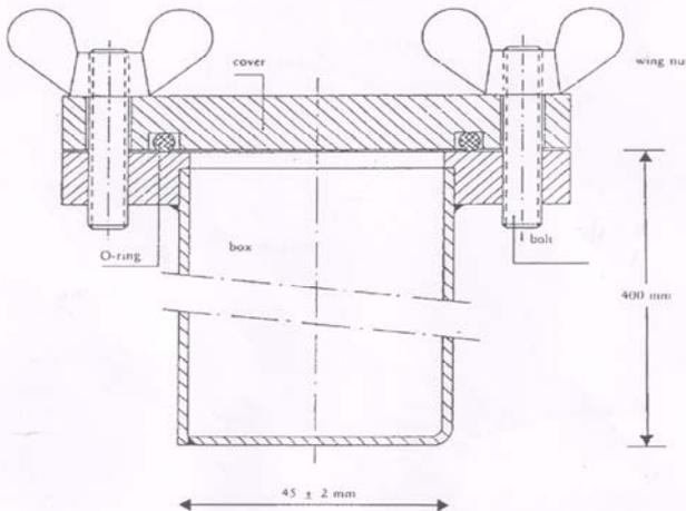
Figure 3 - Metallic box for thermal cycles.
