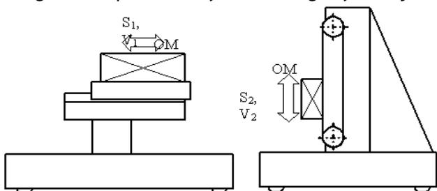
Figure 3. Input values for the design of translation unit
