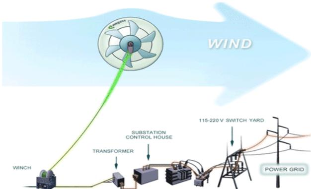
Figure 2. Schema of wiring connection for the M.A.R.S. [2]
