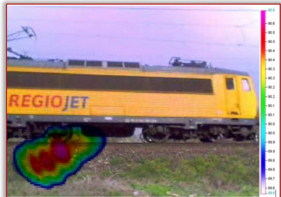
Figure 8. Acoustic image - rolling noise, 80 Hz
