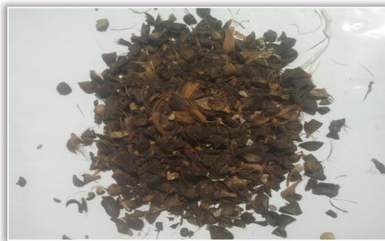
Figure 1: Palm kernel Shell (Source: Mayowa *et al.*, 2015)
