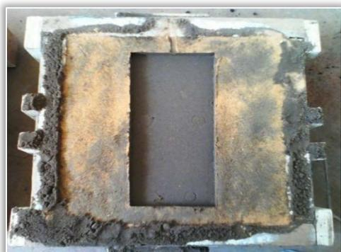
Figure 2: Sand mould without chill
