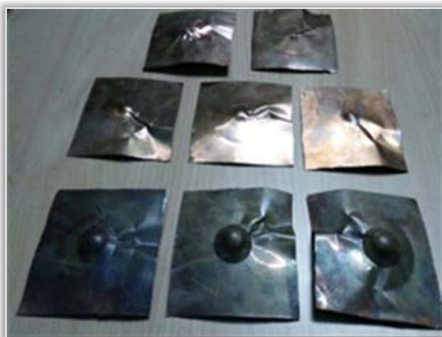
Figure 2. Erichsen cupping test – copper foil
