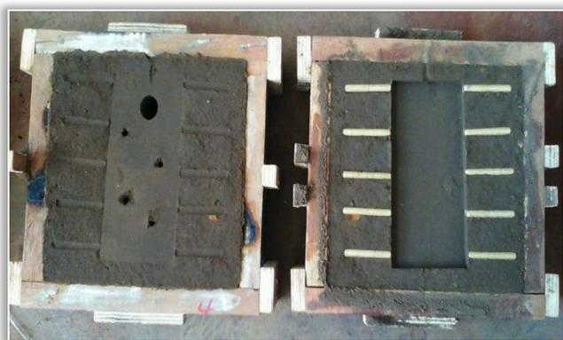
Figure 1: Sand mould with chills
