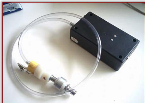
Figure 1: Personal sampling unit with pump
