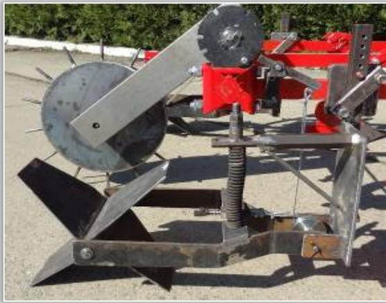
Figure 4 – Device of forming compartmented furrows
