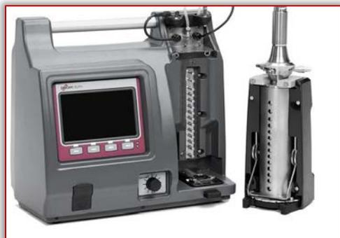
Figure 3: Dekati ELPI – cascade impactor
