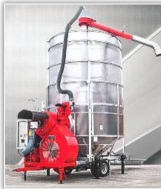
Figure 4 - PEDROTTI trailed vertical dryer [11]
