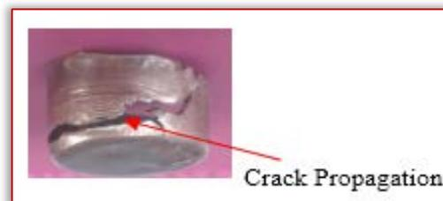
Figure 5. Failure by crack propagation
