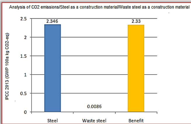
Figure 1. Analysis of kg CO<sub>2</sub> emissions using steel as construction materials and using waste steel in the construction processes [4]
