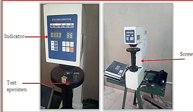
Figure 1: Brinell hardness test of test material
