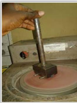
Figure 6: Test specimen under wear test
