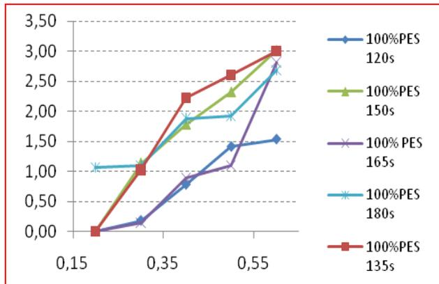
Graph 1: Dependence of strength (y axis) on amount of added water (x axis) for 100% polyester
