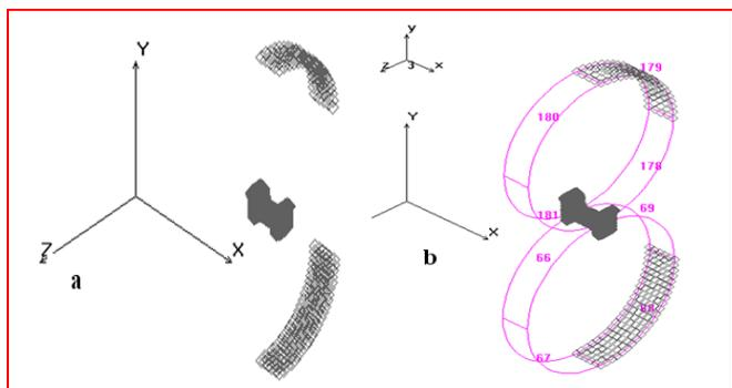
Fig. 3. The rolling roll cooling diagram, without displaying the surfaces the cooling water is applied on (position a) and displaying them (surfaces 68 and 179) (position b)
