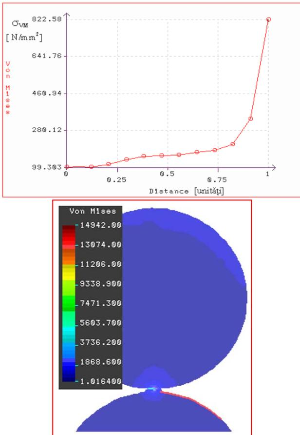
Fig. 7. The variation of Sigma Von Mises strains
