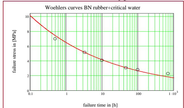
Figure 8. Wöhler's curve for PI – first concentration of water
