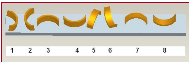
Figure.3 Resting orientations of brakeliner
