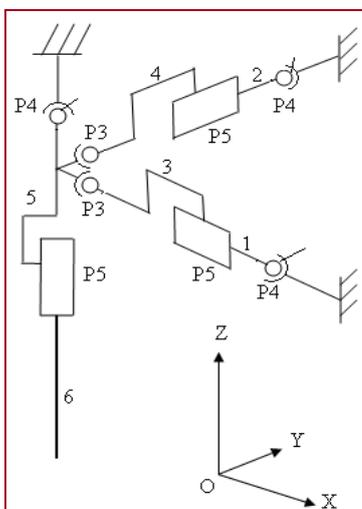
Figure 5. Kinematical chain of micro-manipulator with 3 DoF
