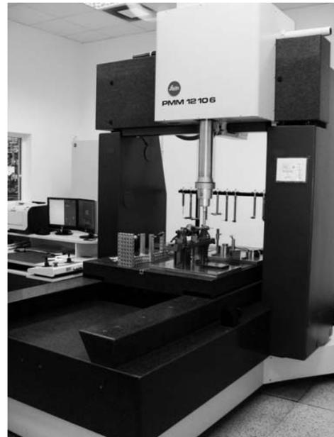
Figure 3 – Tactile coordinate measuring machine Leitz PMM 12.10.6
