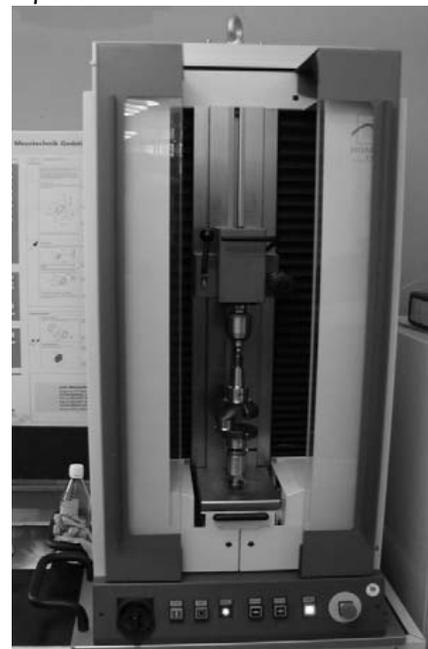
Figure 4 – Optical coordinate measuring machine Hommel Opticline Contour 514
