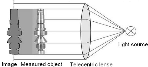
Figure 2 – Measurement principle of optical telecentric system
