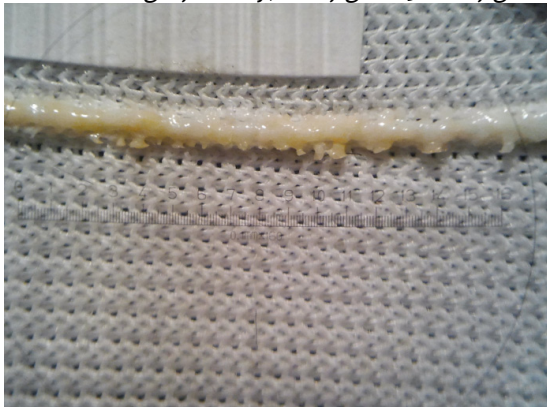
Figure 5 - Laser welded sample, line energy 4.8 kJ/m
