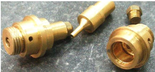
Figure 5: Assembled and disassembled of a Manufactured Injector
