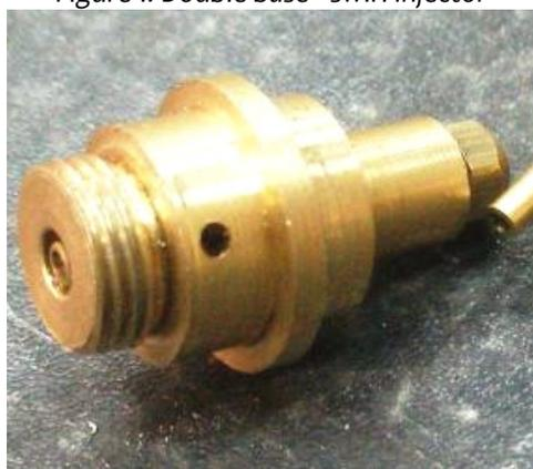
Figure 2: A Manufactured Injector
