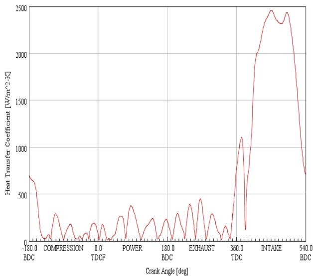
Figure 9. Heat transfer coefficient in intake port at 4500 rpm
