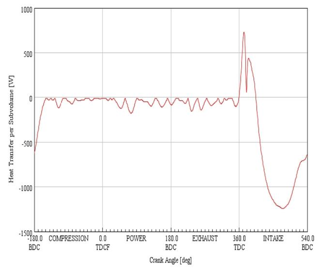
Figure 17. Fluid to wall heat transfer rate in intake port at 4000 rpm
