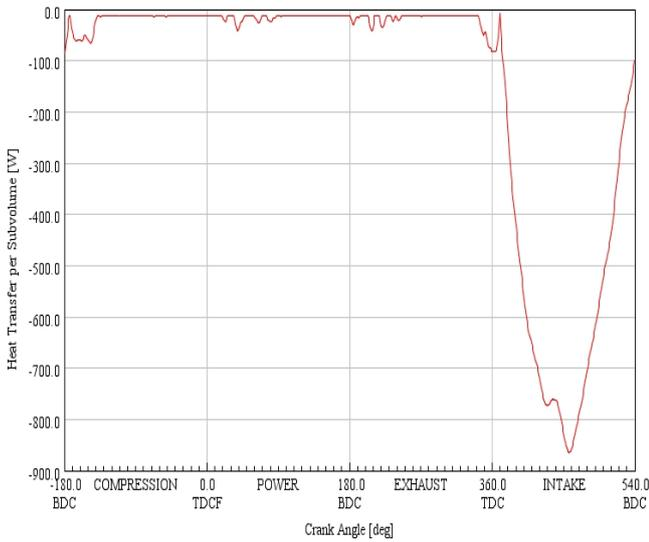
Figure 13. Fluid to wall heat transfer rate in intake port at 2000 rpm
