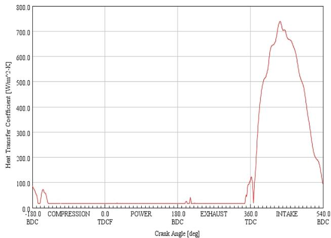
Figure 3. Heat transfer coefficient in intake port at 1500 rpm
