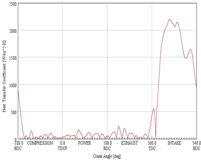
Figure 7. Heat transfer coefficient in intake port at 3500 rpm
