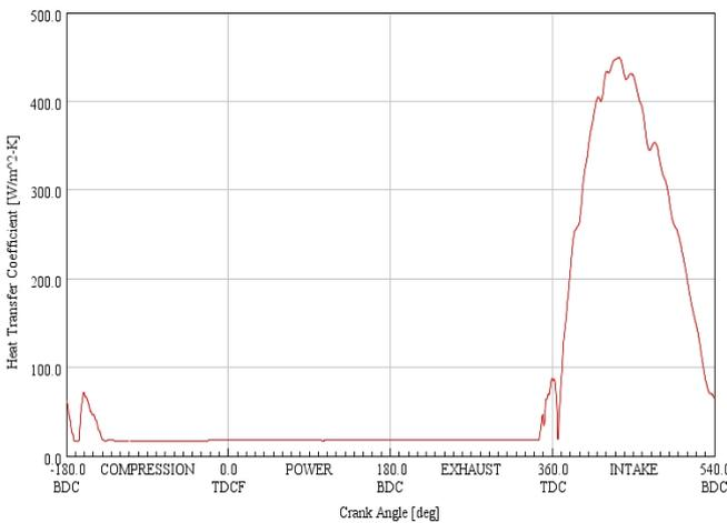
Figure 2. Heat transfer coefficient in intake port at 1000 rpm
