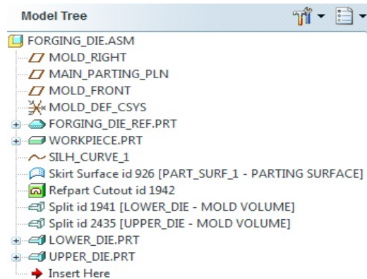
Figure 7. Process tree at cavity creation by “mold cavity mode” method
