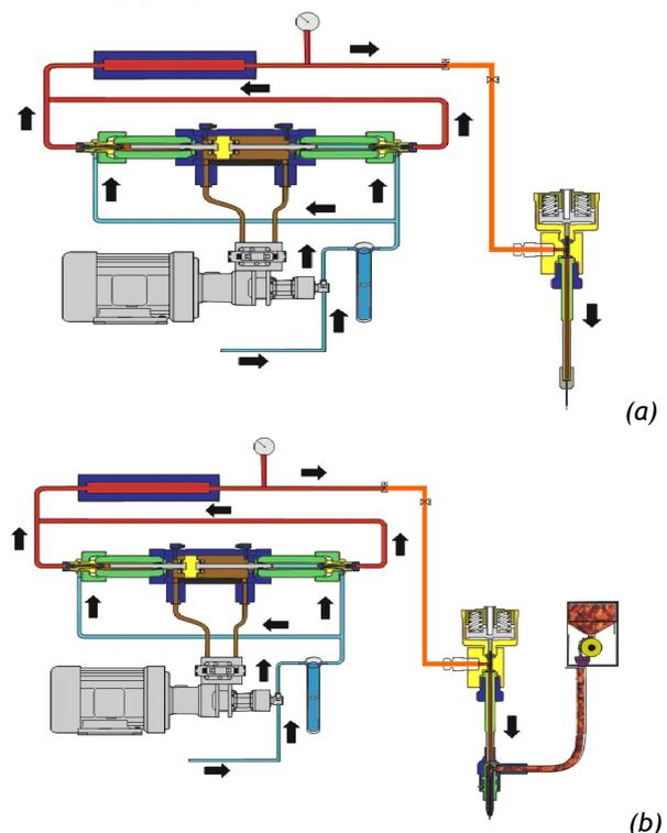
Figure 1: Schematic representation of the principles of water jet cutting and hydroerosion cutting: (a) WJM (hydrodynamic water jet) and (b) AWJM (hydroabrasive water jet)
