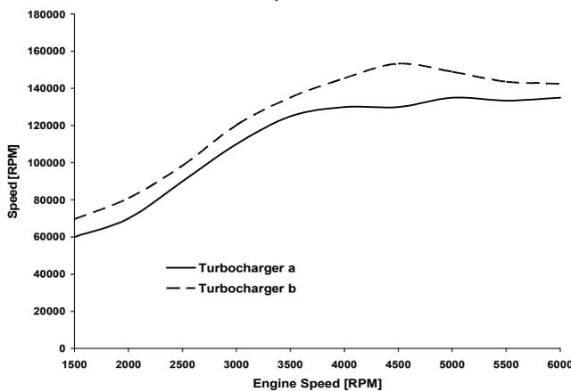
Figure 15. The turbocharge round across two engines at full load state
