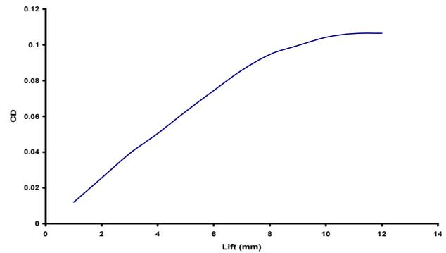
Figure 2. The discharge coefficients in the valve inlet
