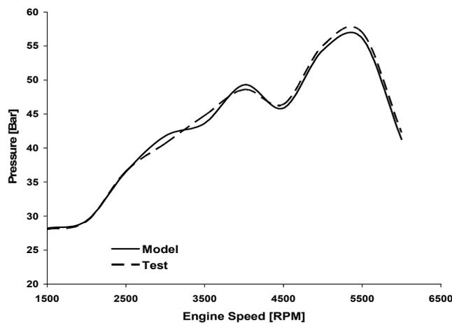
Figure 7. Values for maximum pressure cylinder gasoline engine at various speeds
