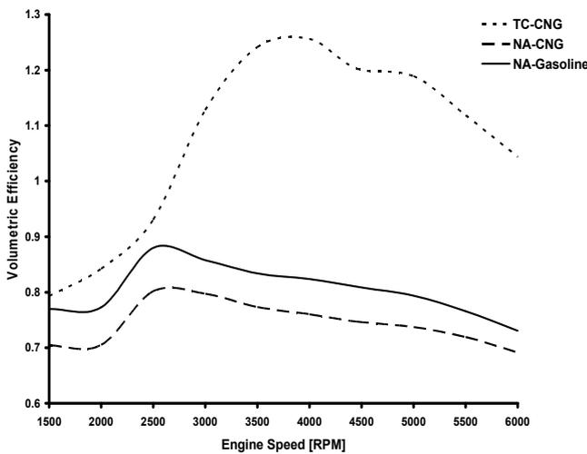
Figure 18. XU-7 engine volumetric efficiency versus engine speed for both normal breathing and overfeeding
