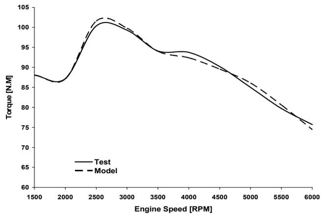
Figure 10. CNG engine brake torque at various speeds
