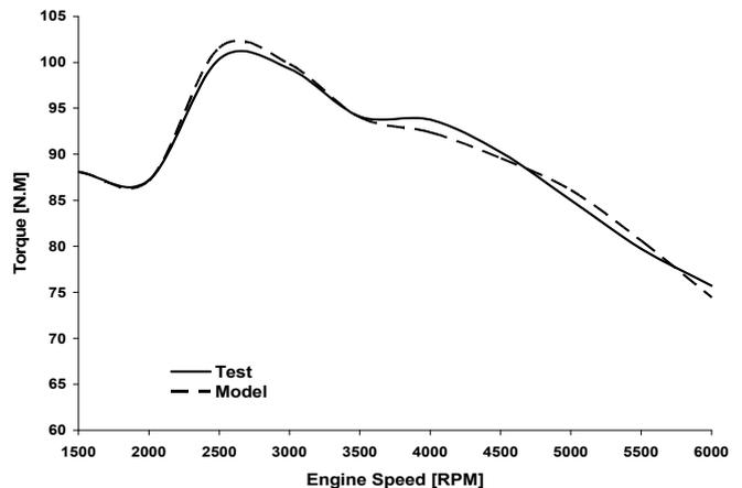
Figure 11. Gasoline engine brake torque at various speeds
