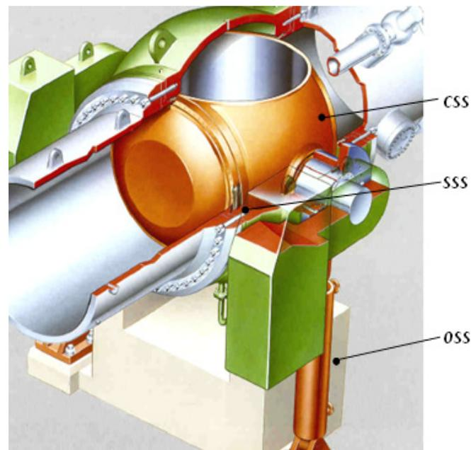
Figure 1. The spherical valve subsystems
