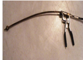
Figure 4. Exhaust gas probe
