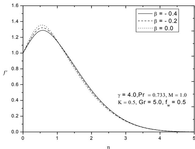
Figure 3. Velocity profiles for different values of  $\beta$
