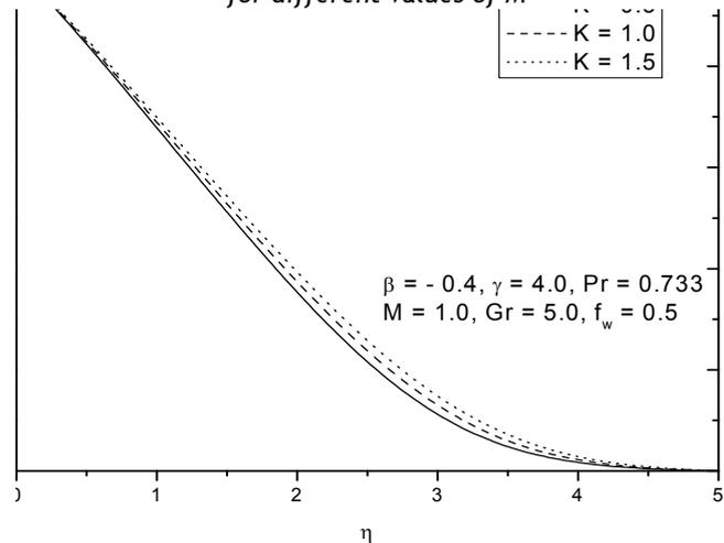
Figure 8. Temperature profiles for different values of  $K$
