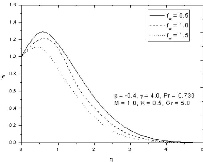
Figure 6. Velocity profiles for different values of  $f_w$
