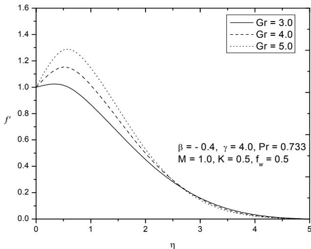
Figure 5. Velocity profiles for different values of  $Gr$
