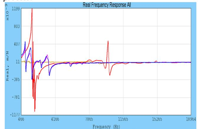
Figure 11. FRF characteristics of measuring system. Blue and purple line is corresponds to tool. Red line is work-piece in the X direction (10 mm thickness). Brown line is work-piece in the Y direction (80 mm length).
