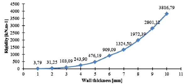
Figure 5. Dependence of wall static rigidity on wall thickness - force in the middle of the wall
