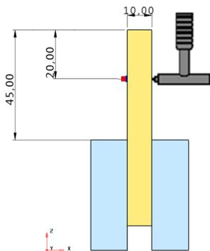
Figure 9. Scheme of FRF measurement of work-piece
