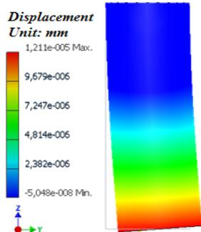
Figure 8. Tool bending in Inventor Pro 2010
