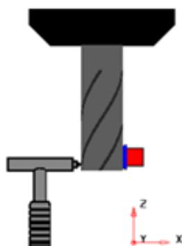
Figure 10. Scheme of FRF measurement of tool
