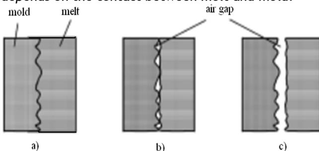
Figure 1. Possible contacts at the melt-mold interface:
