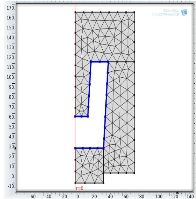
Figure 4. Mesh of the mold assembly consisting of 265 elements
