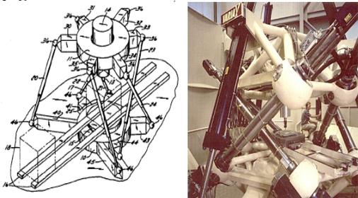
Figure 3.1 Example of parallel robot manipulator, Patent US 5388935: VARIAX machining center,
