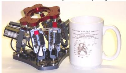
Figure 3.14 Parallel micro robot [52]
