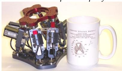
Figure 3.14 Parallel micro robot [52]
