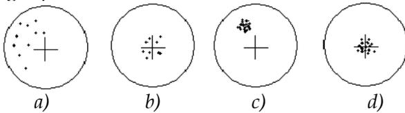
Figure 1.5. a) low accuracy, low repeatability b) high accuracy, low repeatability c) low accuracy, high repeatability d) high accuracy, high repeatability
