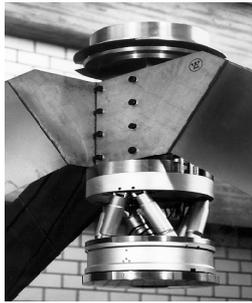
Figure 3.3 Application of parallel robots for fine positioning UKIRT (United Kingdom Infrared Telescope), collaboration between Royal Observatory Edinburgh and Max-Planck-Institut für Astronomie Heidelberg [61]
