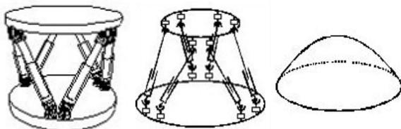
Figure 1.3 Principle, kinematic chain and workspace of parallel robot
