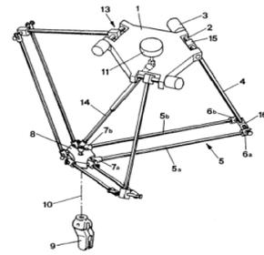
Figure 3.16 Schematic of the Delta robot (from US patent No. 4,976,582) [51]
