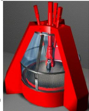
Figure 3.10, Hybrid parallel-serial robot Tricept 805 tripod and a complete machining center [42]
