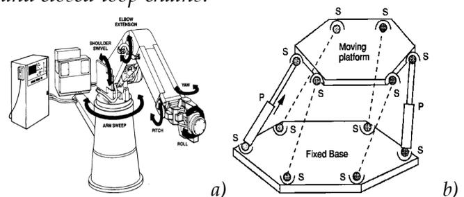
Figure 1.1 a) Serial robot (manipulator) b) parallel manipulator
