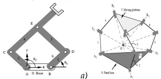
Figure 1.4 a) Planar parallel manipulator b) spherical parallel manipulator
