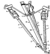
Figure 3.20 3-DOF Parallel kinematic robot Tricept (US Patent No.: US 4,732,525) [51]
