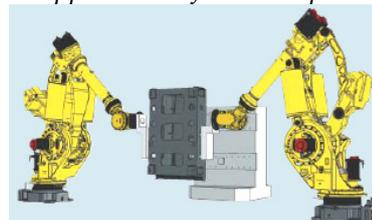
Figure 2.8 Application of two robots in handling heavy objects (materials) [56]
