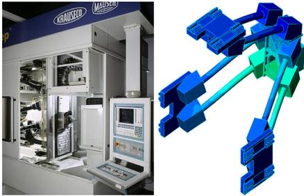
Figure 3.18 The Quickstep 3-axis machining center and Quickstep's kinematic structure [58]
