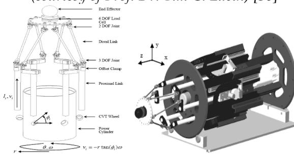
Figure 3.13 Cobotic parallel platform [17]
