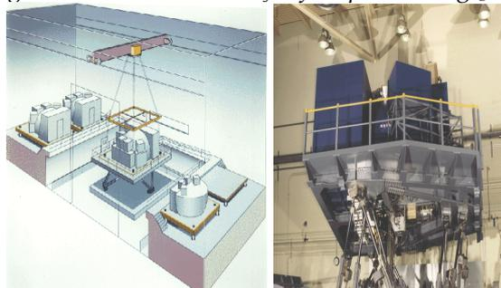
Figure 3.5 Application of parallel robots as simulators NASA LARC-simulator [61]
