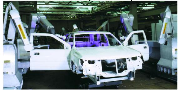
Figure 2.1 Spray painting robots [57]
