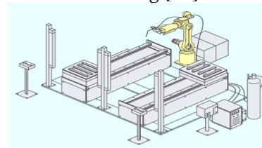
Figure 2.5. Application of robot in welding process [56]
