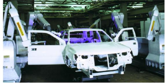
Figure 2.1 Spray painting robots [57]
