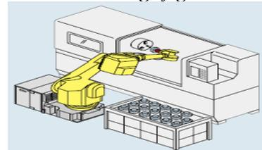
Figure 2.4 Robot application in machine loading and unloading [56]
