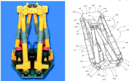
Figure 3.19 A FANUC parallel robot F-200iB [57] (US patent No. 5987726) [51]
