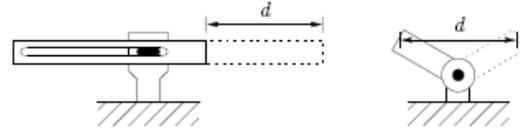
Figure 1.6 Linear vs. rotational link motion.
