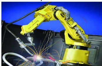
Figure 2.3. Arc welding robot [57]
