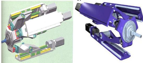
Figure 5.1. Sprint Z3 parallel kinematic tool head [54]
