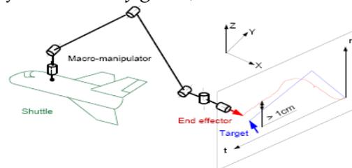
Figure 2.2. Serial space robotic manipulator [1]
