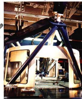
Figure 3.8 Side and top view, solid model and photo of Ingersoll Octahedral Hexapod machine tool installed at NIST [16]
