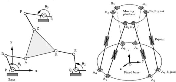
Figure 3.2 a) planar parallel robot manipulator b) spatial parallel robot manipulator
