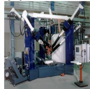
Figure 3.9 Hexapod parallel robot based machine tool [6]
