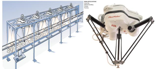
Figure 3.7 Ultra-fast pick and place robot ABB-Flex Picker IRB 340 [50]
