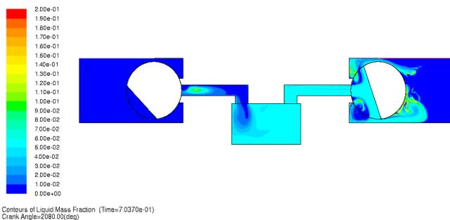
Figure 6. Weight ratio process of aqueous phase in the model for selected rotation angle
