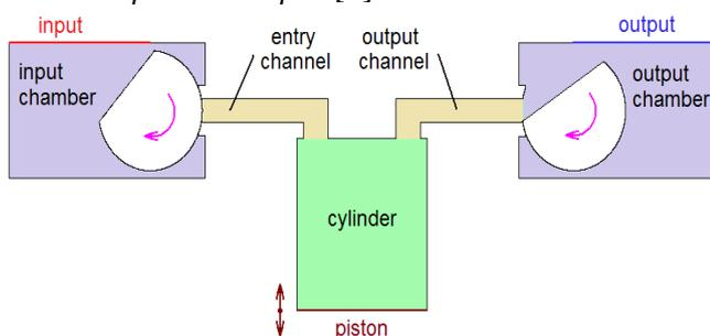
Figure 1. Boundary conditions setting and computational areas labeling of simplified 2D model geometry
