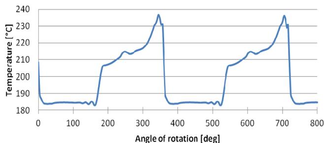
Figure 4. Example of cylinder average temperature course (load time 5°)
