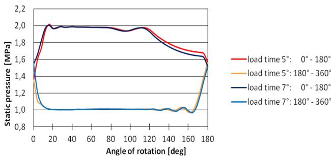
Figure 5. Indicator diagrams for  $p_{in} = 2\text{MPa}$  and  $p_{out} = 1\text{MPa}$ ; load times  $5^\circ$  and  $7^\circ$
