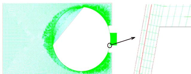
Figure 2. Computational mesh in the input chamber region with auxiliary view of slot area
