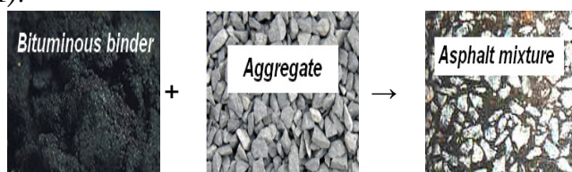
Figure 1. Scheme of creating of asphalt mixture
